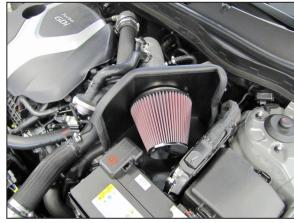
20. Install the K&N® air filter and secure with the provided hose clamp.
