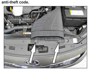
2. Remove the two bolts that secure the fresh air intake scoop to the core support and then remove the fresh air intake scoop from the vehicle.
