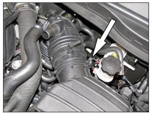
4. Loosen the hose clamp securing the intake hose to the air box.
